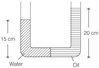
Pressure due to water column of height 15 cm = Pressure due to oil column of height 20 cm
