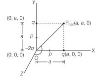
The resultant dipole moment will be directed along *OP* where coordinate of  $\mathbf{p}_{net}$  is given by (*a*, *a*, 0). The magnitude of resultant dipole moment is
