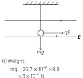
vertically downward, and (ii) Force, F = qE  $= 2 \times 10^{-8} \times 20000$   $= 4 \times 10^{-4} \text{ N}$ In the horizontal direction. So, net tension,  $T = \sqrt{(mg)^2 + F^2}$   $= \sqrt{(3 \times 10^{-4})^2 + (4 \times 10^{-4})^2}$  $= 5 \times 10^{-4} \text{ N}$
