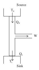
$$1 - \frac{Q_{L}}{Q_{H}} = 1 - \frac{T_{L}}{T_{H}}$$
