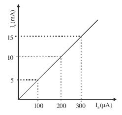
If the input resistance is  $200\Omega$  and output resistance is  $60 \Omega$  the voltage gain in this experiment will be \_\_\_\_\_
