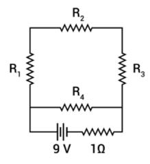
$\begin{aligned} R_1 &= R_2 = R_3 = R_4 = 4\Omega \\ R_{eq} &= 3\Omega + 1\Omega = 4\Omega \\ R_{eq} &= 4\Omega \end{aligned}$
