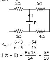
at t =  $\infty$ , inductor is replaced by plane wire, so circuit will look like this at t =  $\infty$
