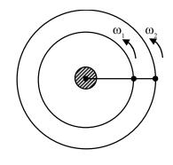
$T_1 = 1$  hour  $\Rightarrow \omega_1 = 2\pi$  rad/hour  $T_2 = 8$  hours
