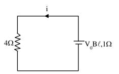
$$i = \frac{V_0 B \ell}{4+1} \implies V_0 = \frac{5(2mA)}{5 \times .2} = 10^{-2} \text{ m/s} = 1 \text{ cm/s}$$
