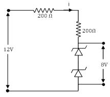
Solution:(40)  $i = \left(\frac{12-8}{200+200}\right) A = \frac{4}{400} = 10^{-2}A$ Power loss in each diode = (4)(10<sup>-2</sup>)  $W = 40 \ mW$
