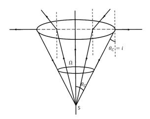
The portion of light escaping into the air from the liquid will form a cone. As long as the angle of incidence on the liquid – air interface is less than the critical angle, i.e.  $i < \theta_c$ , the light rays will undergo refraction and emerge into the air.
