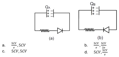
Solution:(a) Maximum charge on capacitor = 5*CV* is forward biased and (b) is reverse biased For case (a)  $q = q_{max}(1 - e^{\frac{-t}{RC}}) = 5CV$   $Q_A = 5CVe^{-1}$ For case (b)  $Q_B = 5CV$
