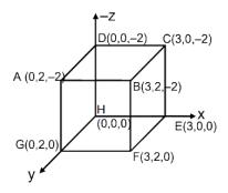
Solution: (-40) Electric flux through a surface is  $\phi = \int \vec{E} = d\vec{A}$ For surface *ABCD*,  $d\vec{A}$  is along  $(-\hat{k})$ So, at all the points of this surface,
