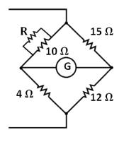
$$\frac{10 \text{ R}}{10 + \text{R}} \times 12 = 15 \times 4 \Rightarrow \text{R} = 10 \Omega$$
