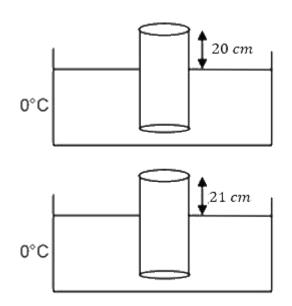
Since the cylinder is in equilibrium, it's weight is balanced by the Buoyant force.
