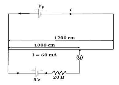
Assume the terminal voltage of the primary battery as  $V_p$ . As long as this potentiometer is operating on balanced length,  $V_p$  will remain constant.
