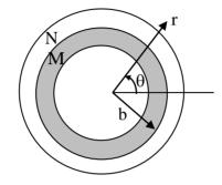
Similarly  $(u_r^N, u_{\theta}^N)$  and  $(\sigma_{rr}^N, \sigma_{\theta\theta}^N)$  denote the radial and tangential displacement and stress components, respectively, in material N. The boundary condition that need to be satisfied at the frictionless interface between the two cylinders are:
