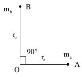
The radii of rotation of the masses  $m_a$  and  $m_b$  are  $r_a$  and  $r_b$ , respectively. The angle between lines OA and OB is 90°. If  $m_a = 10 \text{ kg}$ ,  $m_b = 20 \text{ kg} \text{ r}_a = 200 \text{ mm}$  and  $r_b = 400 \text{ mm}$ , then the balance mass to be placed at a radius of 200 mm is \_\_\_\_\_ kg (round off to two decimal places)
