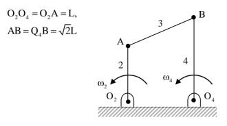
The magnitude of the angular speed of the output link 4 is  $\omega_4$  at the instant when link 2 makes an angle of 90° with  $O_2O_4$  as shown. The ratio  $\frac{\omega_4}{\omega_2}$  is \_\_\_\_\_(round off to two decimal places).
