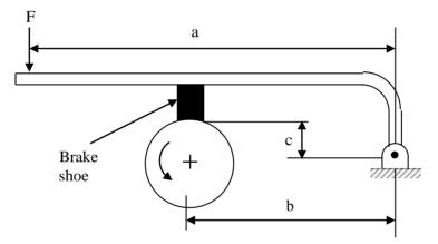
The force applied on the lever F = 100 N as shown in the figure. The drum is rotating anti-clockwise. The braking torque on the drum is \_\_\_\_\_ N-m (roundoff to two decimal places).
