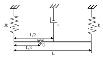
For the system to be critically damped, the ratio  $c / \sqrt{km}$  should be
