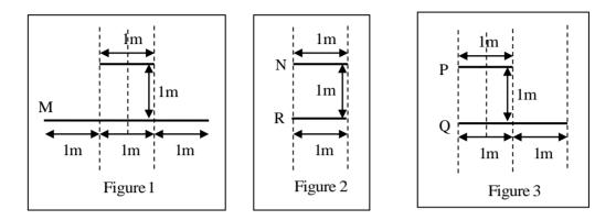
Assume that the values of  $F_{LM}$  and  $F_{NR}$  are 0.8 and 0.4 respectively. The value of  $F_{PQ}$  (round off to one decimal place) is\_\_\_\_\_.
