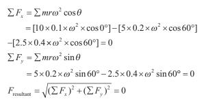
Since, this is a balanced system so, net force on bearing is zero.
