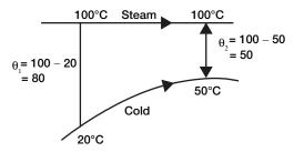
Log Mean Temperature Difference can be calculated as
