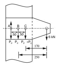
$$P_p = \frac{6}{3} = 2\text{KN}\{P_p = \text{Primary shear force}\}$$
