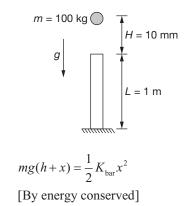
$$K_{\text{bar}} = \frac{EA}{L} = \frac{100 \times 10^9 \times 100 \times 10^{-6}}{1} \text{ N/m}$$
