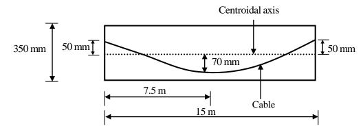
If the cable is tensioned from one end only, the percentage loss (round off to one decimal place) in the cable force due to friction, is \_\_\_\_\_.
