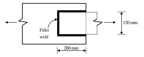
As per Limit State Design is IS 800: 2007, the design capacity (in kN, round off to three decimal places) of the welded connection, is \_\_\_\_\_.
