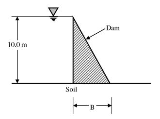
The coefficient of friction between the dam and foundation soil is 0.45. Specific weights of concrete and water are  $24 \text{ kN/m}^3$  and  $9.81 \text{ kN/m}^3$ , respectively.
