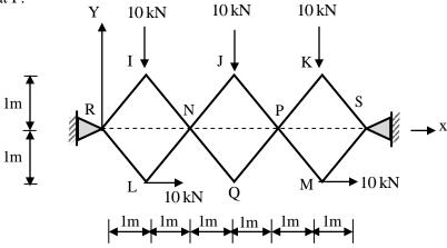
The frame has hinge supports at joints R and S. The loads acting at joints I, J and K are along the negative Y direction and the loads acting at joints L, M are along thepositive X direction. The magnitude of the horizontal component of reaction (in kN) at S, is
