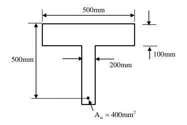
As per IS 456:2000, the limiting depth (in mm, round off to the nearest integer) of the neutral axis measured from the extreme compression fiber, is \_\_\_\_\_.
