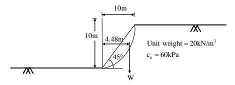
The factor of safety of the slope against slip failure, is
