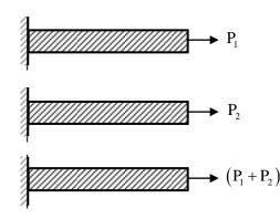
If U is the strain energy stored in the same bar when subjected to an axial tensile force  $(P_1 + P_2)$ , the correct relationship is
