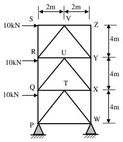
Representing the tensile force with '+' sign and the compressive force with '-' sign, the force in member XW (in kN, round off to the nearest integer), is \_\_\_\_\_.
