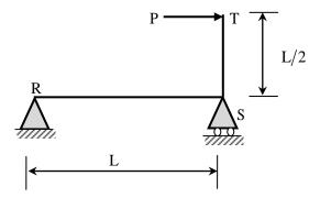
When the structure is subjected to a concentrated horizontal load P at the end T, themagnitude of rotation at the support R, is
