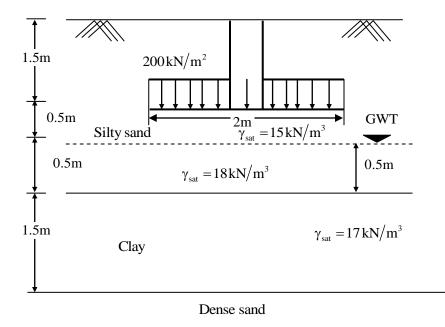
The clay has specific gravity of 2.65 and compression index of 0.3.
