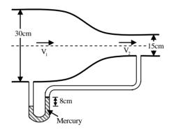
When the water flow, the differential manometer shows a deflection of 8cm of mercury (Hg). The value of specific gravity of mercury and water are 13.6 and 1.0, respectively. Consider the acceleration due to gravity.  $g = 9.81 \text{ m/s}^2$ . Assuming frictionless flow, the flow rate (in m<sup>3</sup>/s, rounded off to 3 decimal places) through the duct is \_\_\_\_\_.
