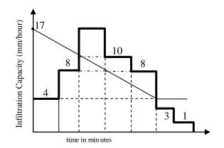
The infiltration capacity at the start of this event (t = 0) is 17mm/hour, which linearly decreases to 10 mm/hour after 40 minutes duration. As the event progresses, the infiltration rate further drops down linearly to attain a value of 4mm/hour at t = 100 minutes and remains constant thereafter till the end of the storm event. The value of the infiltration index,  $\phi$  (in mm/hour, round off to 2 decimal places), is \_\_\_\_\_.
