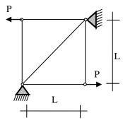
For the loads shown on the truss, the statement that correctly represents the nature of forces in the members of the truss is:
