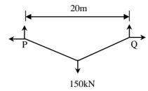
Neglecting the self weight of the cable. The tension (in kN. In integer value) in the cable due to the applied load will be \_\_\_\_\_.
