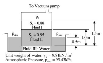
The gauge pressure value (in  $kN/m^2$ . Up to two decimal places) of  $p_1$  is \_\_\_\_\_
