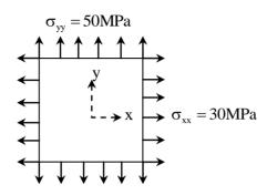
The Young's modulus of the material is  $2\times10^{11} N/m^2$  and the Poisson's ratio is 0.3 if  $\sigma_{zz}$  is negligibly small and assumed to be zero. Then the strain  $\epsilon_{zz}$  is
