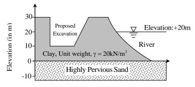
The water level in the adjacent river is at an elevation of +20.0m. Unit weight of water is 10kN/m $^3$ . The factor of safety (up to two decimal places) against sand boiling for the proposed excavation is \_\_\_\_\_\_\_.
