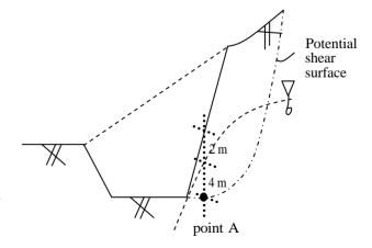
factors of safety against the shear failure at this point, considering the undrained and drained conditions, respectively, would be
