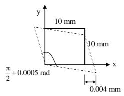
If the shear strain  $\gamma_{xy}$  at this point is expressed as 0.001k (in rad), the value of k is
