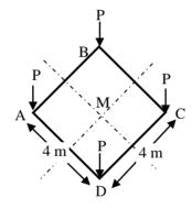
The vertical stress increment (in kPa, up to one decimal place) due to these loads according to the Boussinesq's equation, at a point 5 m right below M, is\_\_\_\_\_.
