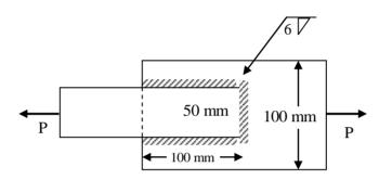
The permissible stresses in the plate and the weld are 150 MPa and 110 MPa, respectively. Assuming the length of the weld shown in the figure to be the effective length, the permissible load P (in kN) is\_\_\_\_\_.
