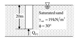
If  $Q_{P1}$  and  $Q_{P2}$  represent the ultimate point bearing resistance of the piles under dry and submerged conditions, respectively, which one of the following statements is correct?
