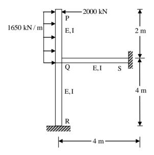
The rotation (in degrees, up to one decimal place) at the rigid joint Q would be\_\_\_\_\_
