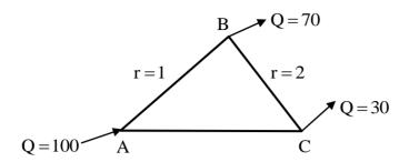
The head loss in each pipe is given by  $h_f = rQ^{1.8}$ , with the variables expressed in a consistent set of units. The value of r for the pipe AB is 1 and for the pipe BC is 2. If the discharge supplied at the point A (i.e., 100) is equally divided between the pipes AB and AC, the value of r (up to two decimal places) for the pipe AC should be\_\_\_\_\_
