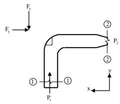
A pressure of 140 kPa is measured at section 1-1. The inlet diameter marked at section 1-1 is  $\frac{27}{\sqrt{\pi}}$  cm, while
