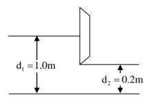
It is observed that the depth of flow is 1.0 m upstream of the gate, while the depth is 0.2 m downstream of the gate. Assuming a smooth flow transition across the sluice gate, i.e., without any energy loss, and the acceleration due to gravity as 10 m/s<sup>2</sup>, the discharge (in m<sup>3</sup>/s, up to two decimal places) passing under the sluice gate is\_\_\_\_\_\_.
