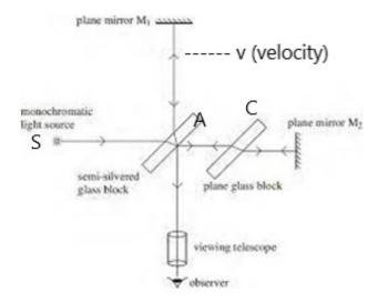
Monochromatic source S is taken and light is made to fall from it on lens combination. The half silvered plate A splits it into two components, one parallel and one perpendicular. The reflected component travels to the mirror M<sub>1</sub> and is reflected back, while the transmitted component is reflected back from M<sub>2</sub>.
