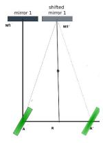
The reflected beams from M<sub>1</sub> and M<sub>2</sub> interfere and the interference fringes are observed through the telescope T.The appararus is arranged to move along the direction of the earths orbit around the sun, with velocity of earth v, this whole apparatus was floated on mercury and was adjusted such that it is always moving along the direction of the earths orbit round the sun.
